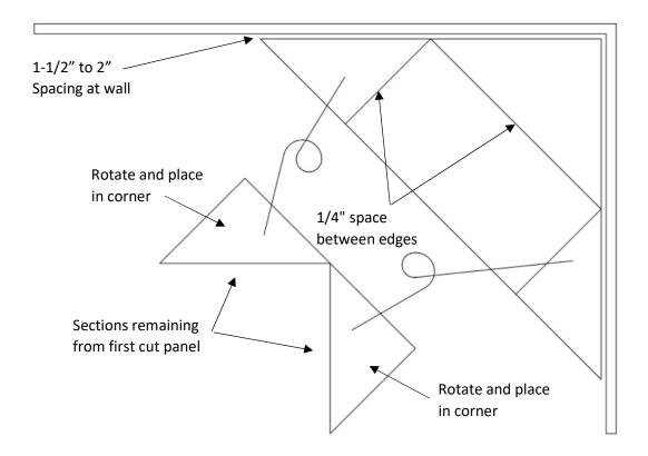
10. As shown below, plywood panels can be cut in this manner to provide starting and ending panels to complete rows.
