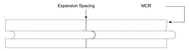
The inclusion of the MCR option can be advantageous as a manner to include expansion spacing for anticipated wood flooring growth after installation.
