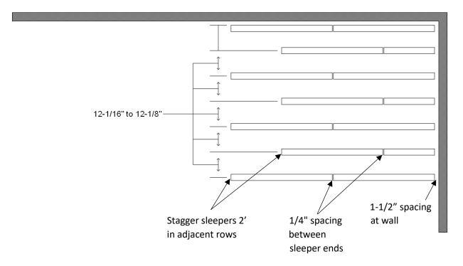
10. Install plywood subfloor layer as shown on following page by alternating 5' and 3' sections when starting rows to offset plywood ends by 2' in adjacent rows, and to offset plywood ends by 12" from sleeper ends.
