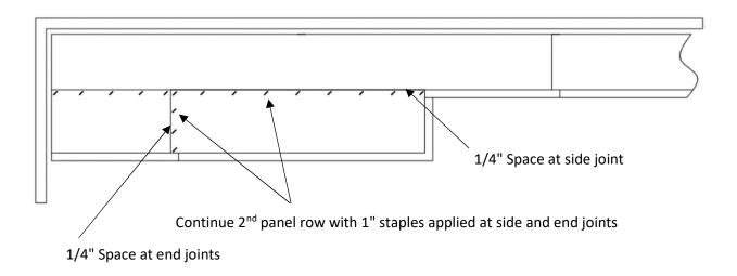
Start remaining odd numbered rows as shown below by removing overhanging end edge. Space panel 1-1/2" from wall and overlap and attach side joint as previously described, with 1/4" spacing from adjacent panels.
