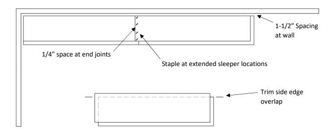
6. Start second panel row and all even numbered rows as shown below by cross cutting full panel 48" measured off of bottom subfloor layer. Offset side edge 1/4" from adjacent subfloor panel and attach overlapping side edge to adjacent panel with 1" subfloor staples applied 12" on center including at ends.
