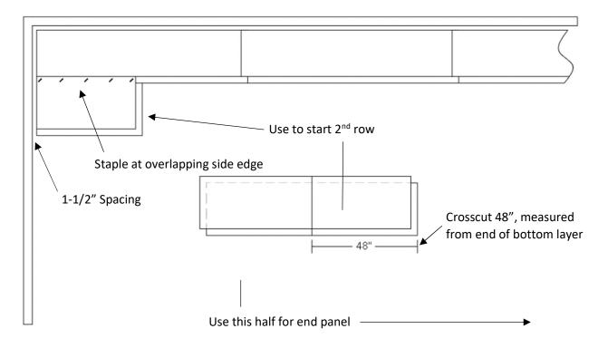
7. Continue second panel row with full subfloor panels with panel edges offset 1/4" from adjacent panels. Fasten panel side edge and end edge as illustrated below with minimum four fasteners at end joints and spaced 12" on center at side joints.
