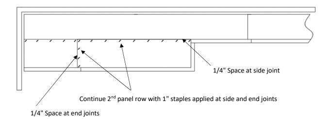
8. Start remaining odd numbered rows as shown below by removing overhanging end edge. Space panel 1-1/2" from wall and overlap and attach side joint as previously described, with 1/4" spacing from adjacent panels.
