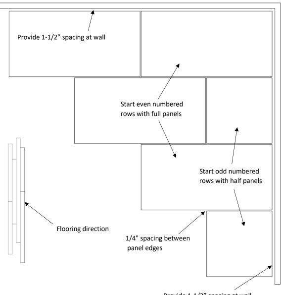
Provide 1-1/2" spacing at wall
