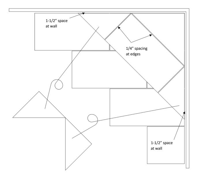
12. Provide nominal 1-1/2" spacing at walls and nominal 1/4" spacing between panel edges.
