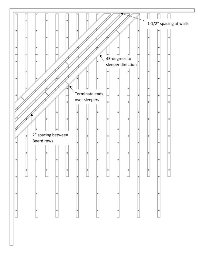
15. As shown on the following page, do not align end joints of upper subfloor boards adjacent to each other over sleeper intersections.
