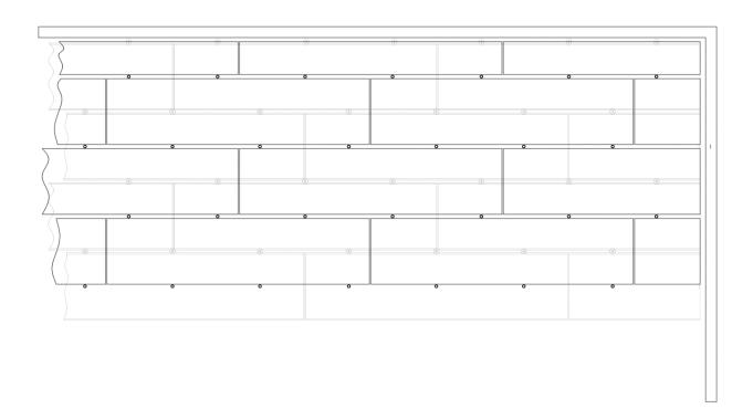
• To reduce waste, partial panels from completion of previous rows can be acceptably used to start panel rows provided that panels are minimum 16" in length and provided that panel ends and anchors are offset by a minimum of 12" from panel ends of adjacent rows.
