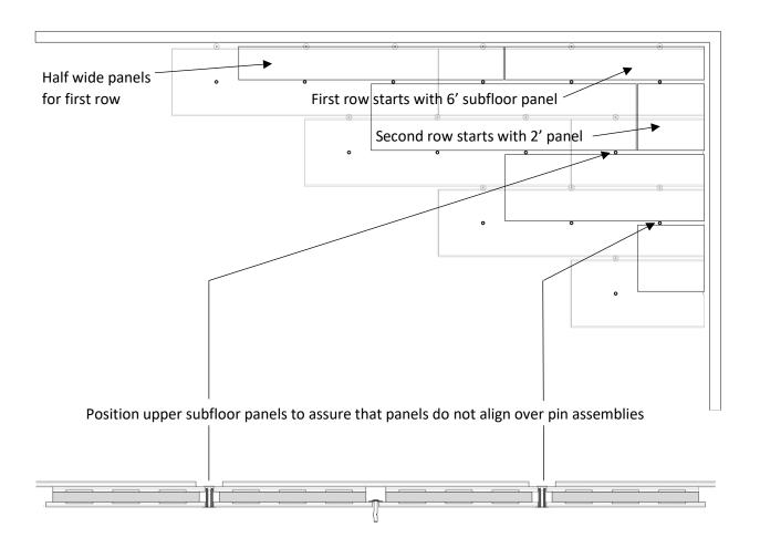
12. Continue subfloor installation as shown below by staggering upper and lower panel ends and by maintaining an offset pattern of concrete anchors.
