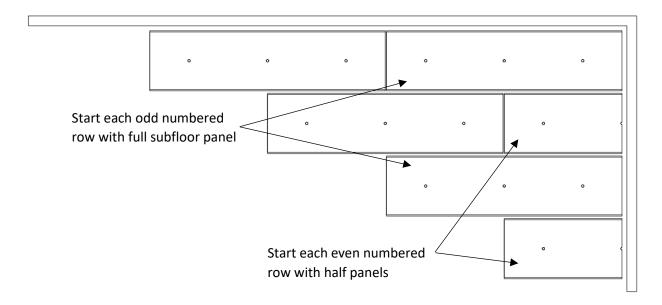
6. Anchor subfloor panels to concrete as indicated below with anchorage pins and washers in direct alignment to the right of subfloor panel pin assemblies when working along each row.
