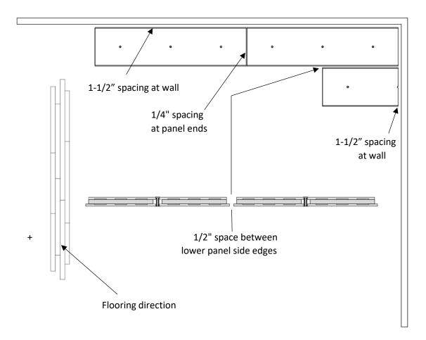
4. Include 1/4" spacing between panel ends as shown above.
