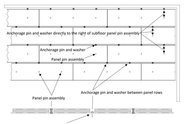
Drill with 1/4" masonry bit and only drive until washer makes contact with subfloor surface
