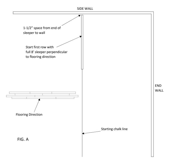
1. Align first sleeper with chalk line as shown above. The inclusion of a semi-clear surface vapor barrier/retarder can allow identification of chalk line when snapped directly on the concrete surface rather than on top of the vapor retarder.
