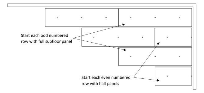
6. Anchor subfloor panels to concrete as indicated below with anchorage pins and washers in direct alignment to the right of subfloor panel pin assemblies when working along each row.
