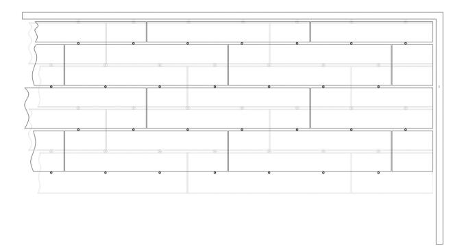
• To reduce waste, partial panels from completion of previous rows can be acceptably used to start panel rows provided that panels are minimum 16" in length and provided that panel ends and anchors are offset by a minimum of 12" from panel ends of adjacent rows.
