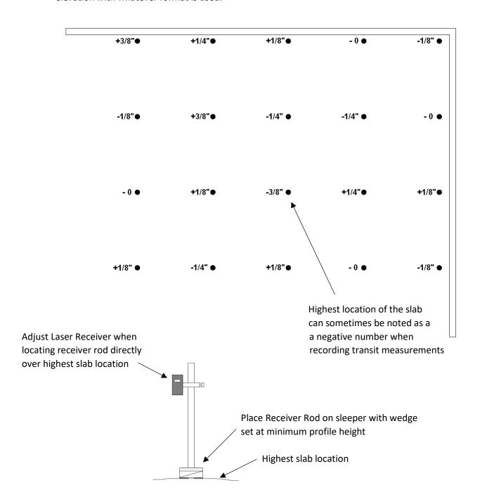
3. As shown below, padded profile blocks are adjusted in relation to the concrete slab elevation. Deck type wood screws are required in three available option lengths along with the application of wood glue on the wedge surface before fastening.
