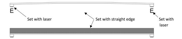
7. Without using laser, apply slight hand pressure to assure previous assembled wedges are in contact with the concrete slab when setting inner wedge locations (X).
