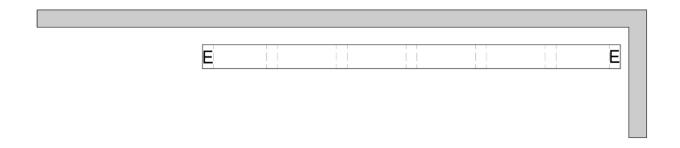
6. With two end wedges installed, use 8' straight edge placed from end (E) to end (E) to assure sleeper surface is flat.
