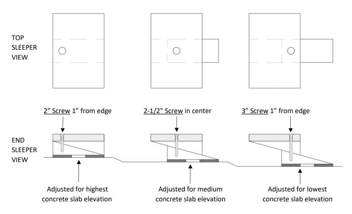
4. As shown below, install first ReClaim sleeper perpendicular to flooring direction with side spaced 4" from wall and end spaced 1-1/2" from wall.
