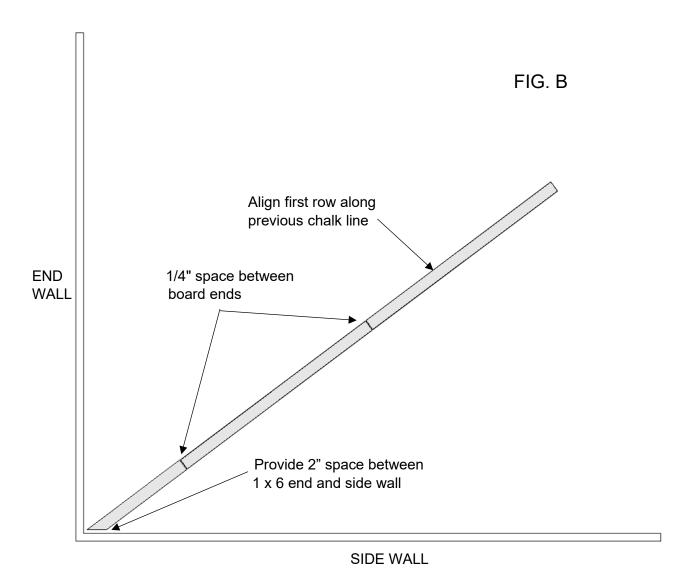
2. Align first 1 x 6 row along chalk line as shown above with 2" spacing provided between
