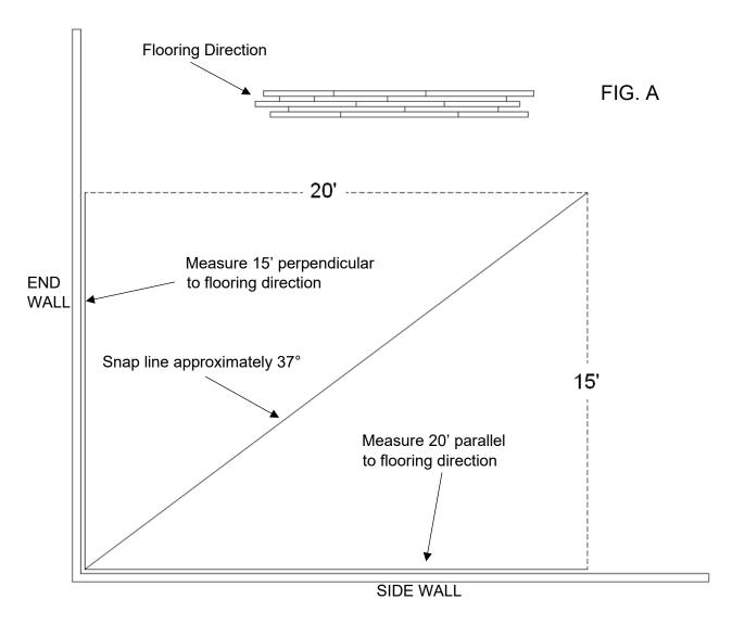
1. Define lower subfloor direction with chalk line as shown above located 20' out from corner along wall parallel to flooring direction to 15' out from corner along wall perpendicular to flooring direction. This creates an approximate 37-degree angle.
