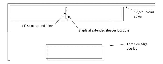
6. Start second panel row and all even numbered rows as shown below by cross cutting full panel 48" measured off of bottom subfloor layer. Offset side edge 1/4" from adjacent subfloor panel and attach overlapping side edge to adjacent panel with 1" subfloor staples applied 12" on center including at ends.
