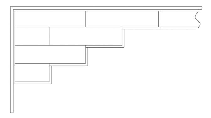
• To reduce waste, partial panels from completion of previous rows can be acceptably used to start panel rows provided that panels are minimum 16" in length and provided that panel ends are offset by a minimum of 12" from panel ends of adjacent rows.
