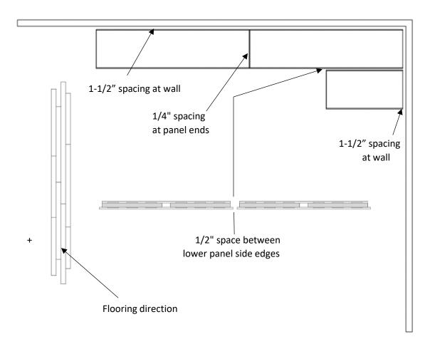
4. Include 1/4" spacing between panel ends as shown above.
