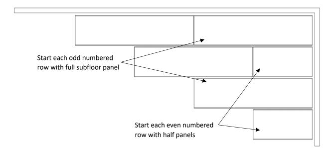
6. Secure subfloor panels to concrete with anchors and washers spaced and located as shown below to create a diamond pattern.
